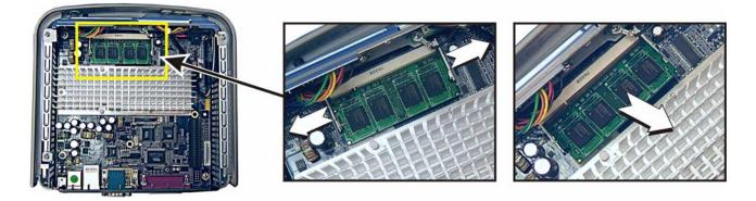
6. Install the 512-MB RAM module, label facing down, into the location of the original module at the same angle, and then press module's raised edge downward until it snaps in place.
